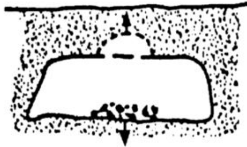
(a) CAVITY COLLAPSE
